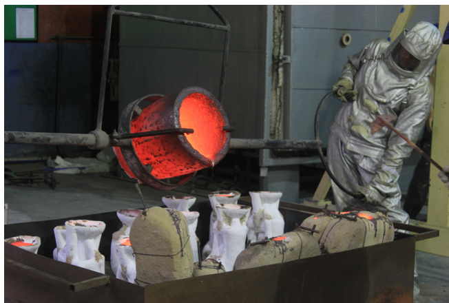
Pouring of the silicon bronze into ceramic shell molds.
